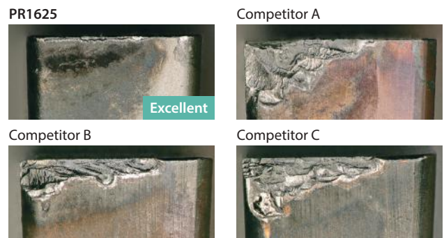
Cutting Conditions : V_c = 140 m/min, f = 0.12 mm/rev, Insert width 3mm Workpiece : SCM440 with 16 Slots External Grooving (Heavy Interruption)
