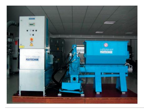
A BrikStar V is configured as a press unit with separate hydraulic system, electrical panel (including PLC controls) and flange for connecting a screw feeder and trough; but without hopper and agitator or hopper and walking floor. This press is the ideal solution for very specific requirements; otherwise it has an identical performance to a BrikStar CM. We would welcome the opportunity of discussing with you how a BrikStar VM could be integrated into your production process.
